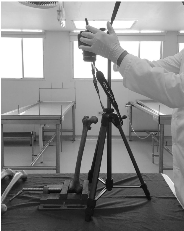
Fig. 2 Positioning of the femur and of the equipment used for photographing the specimens
